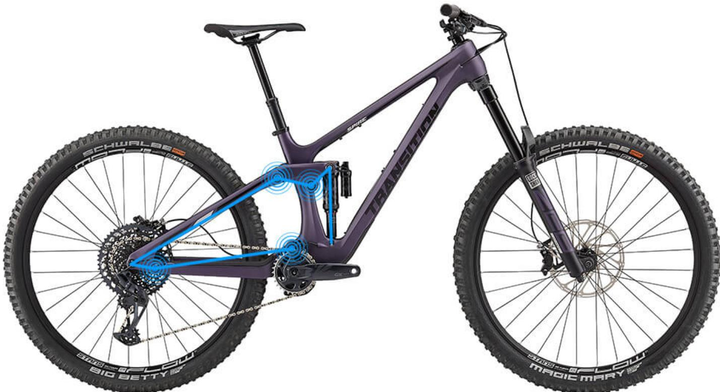
With nearly 23% progression and the most current evolution of our GiddyUp suspension kinematic, the Spire has an excellent balance of support and small bump sensitivity. Anti-squat is tuned to enhance pedaling performance and provides a platform to push against when pumping, without sacrificing a bottomless feel when needed.
