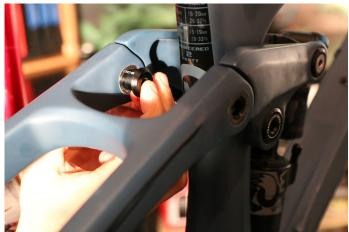
Step 31 continued: Add a small amount of grease to the outsides of all four bearings located towards the rear of the seat stay to help keep the bearing shields stay in place. Then carefully slide the chain stay over the seat stay. Be mindful to not pull up on the seat stay as it will potentially damage the seat stay / rocker junction.
