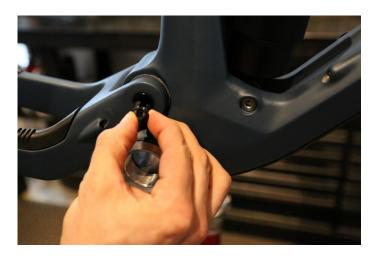
Step 7: Remove the pain pivot from the frame by using an 8mm allen wrench.
