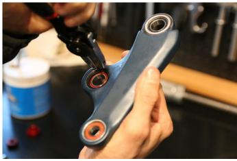
**Step 23:** Grease the main pivot bearing seats and install the main pivot bearings (6903). Install one at a time and make sure to put in the bearing spacer before installing the second bearing.
