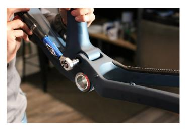
Step 27: Install the main pivot screw, spacer, and taper nut. Apply grease to the main pivot taper nut, and blue Loctite on the threads of the main screw after the taper nut is installed.
