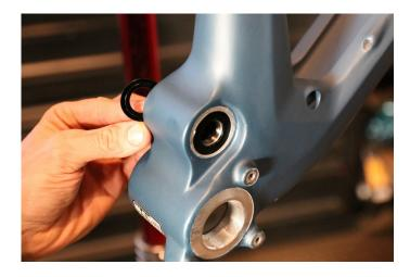
**Step 26:** Grease the shaft of the main pivot, carefully attach the chain stay to the bike. It's helpful to hold onto the bearing shields when re-installing the chain stay.
