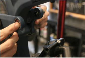
**Step 10:** Remove the lower shock bolt and shock from the frame. You'll need 2, 5mm allen wrenches.
