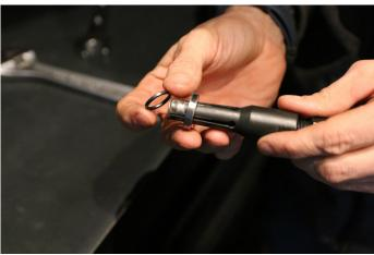
**Step 17:** Now that you've removed the outer bearing, you can push the inner bearing out. Then repeat steps 15-17 on the other side of the seat stay.
