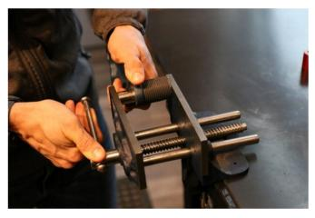
Step 15 continued: Make a note of the bearings and snap rings orientation, there are three different sizes.
