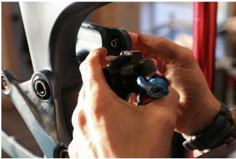
Step 30 continued: Snug down the shock bolts using a 5mm allen wrench. Once snug use a torque wrench and tighten to 12Nm. Now you can torque the lower shock bolt to 10Nm.
