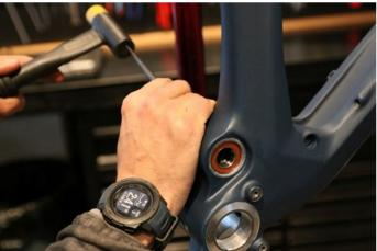
**Step 13:** Remove the spacer and tap the remaining main pivot bearing out of the frame. Making sure to alternate where you're placing the punch to ensure a straight and smooth removal.
