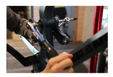
**Step 29:** Install the shock, installing the lower shock bolt first. Make sure to grease the shaft and add blue Loctite to grease to the inside and outside of both forward rocker the inside of the female end. You'll need two 5mm allen wrenches to snug the bolt down. Torque to spec (10Nm) after the upper shock bolts are installed.
