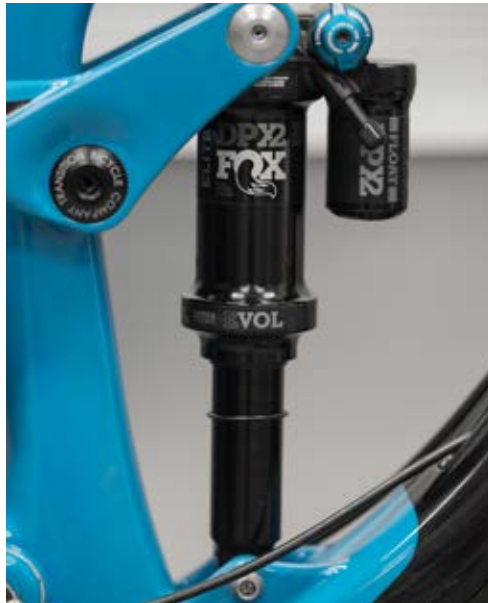
O-ring at proper sag for Sentinel 20mm
