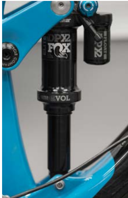
O-ring at top of shock shaft seal
