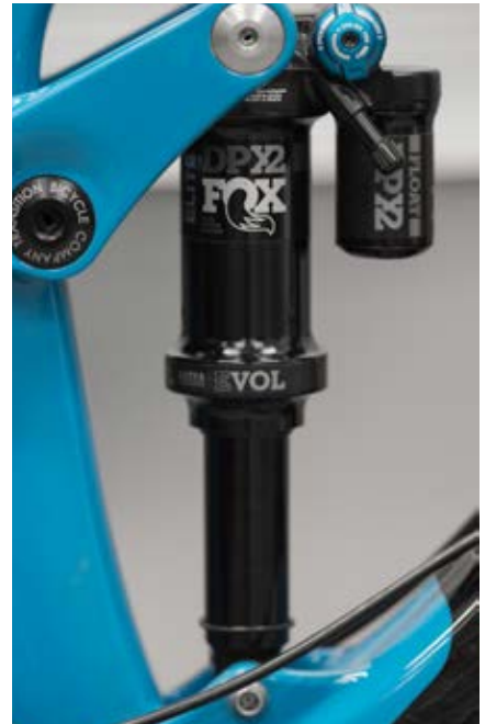
*Shock utilizing full travel with proper sag setup
