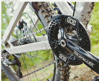
↑ e*thirteen's SRS+ guide does a good job of keeping the chain in check
