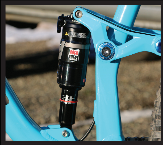
O-ring at proper sag for 35%
