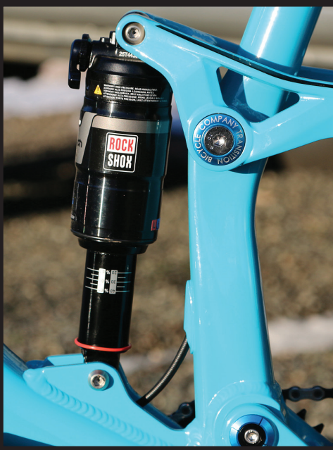
Shock utilizing full travel with proper sag setup
