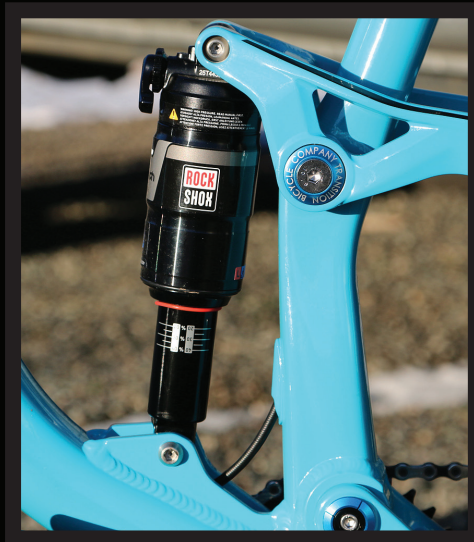
O-ring at top of shock shaft seal
