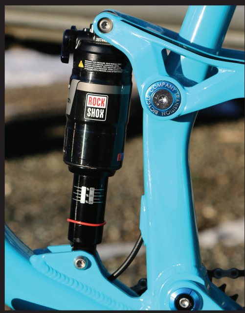
Shock not utilizing enough travel
