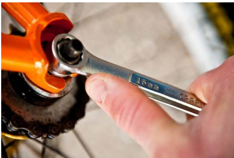
15mm wrench is key to getting this axle tight
