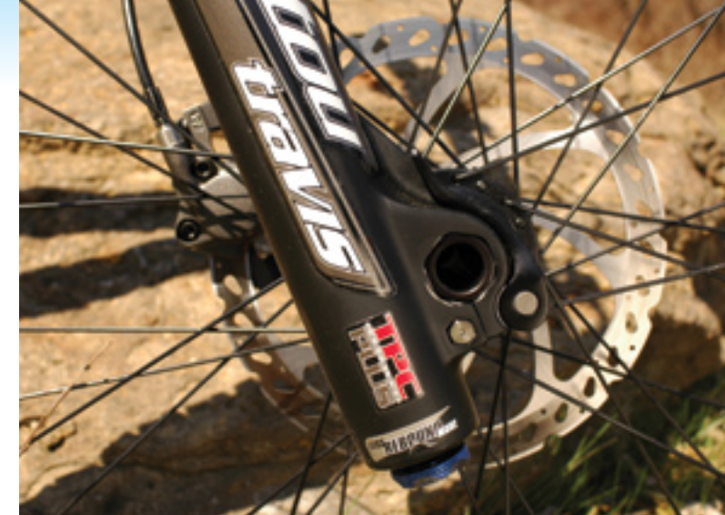
Manitou's quick release 20mm thru axle gives tool-free wheel removal—thanks, Travis!
