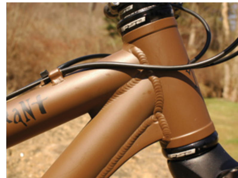
Collars and a thick gusset around the 1.5" head tube.
